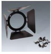
Individually adjustable blades are used to create lamp shielding and tailor the size of a beam pattern to the illuminated area. Blades can be used to create horizontal cut-off (to keep light out of the viewer's eyes) or vertical cutoff (to stop light at the edge of a wall panel or at the intersection of two walls). Finishes: W, SL, BK
