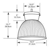
WARNING: Pulse Start Metal Halide lamps are rated for shielded or enclosed fixtures only. Specific lamps can be utilized in open fixtures and require an open rated socket ("OR" option). Consult lamp manufacturers for details.
