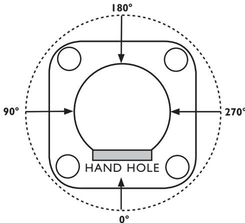
Orientation is measured clockwise from the Hand Hole Center.
