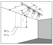
EXAMPLE: With track located 2' from wall and multiple units spaced 2' on center and aimed 75) from horizontal, the illumination on wall 3' from ceiling will be 36 f.c. beneath units and 21 f.c. between units.
