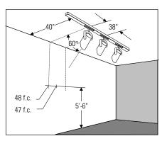
EXAMPLE: With track located 40" from wall multiple units spaced 38" on center and aimed 60J from horizontal, the illumination on wall 5' 6" from floor will be 48 f.c. beneath units and 47 f.c. between units.
