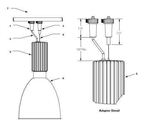
Typical complete installation shown (Power Head and Reflector must be ordered separately).
