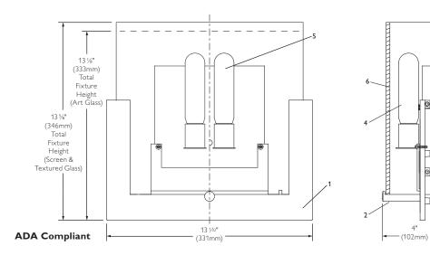
Complete Fixture consists of Lightshield and Backplate Assembly. Order each separately.
