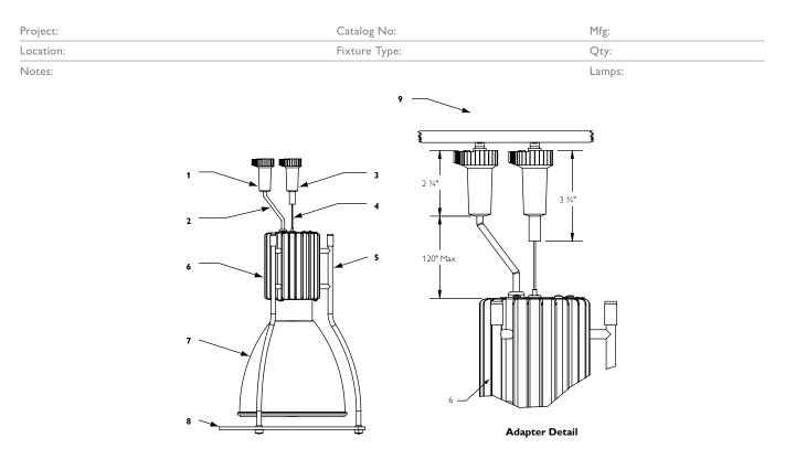
Typical complete installation shown (Power Head, Reflector and Aperture Disk must be ordered separately).
