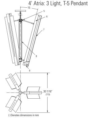
Note: Luminaire can be ordered with or without diffuser shield. Order each separately.
