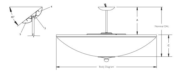
Complete Luminaire consists of Body and Suspension. Order each separately.
