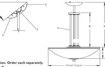
Complete Luminaire consists of Body and Suspension. Order each separately. Multiple Stem Suspension, with Swivel, Basic Canopy.
