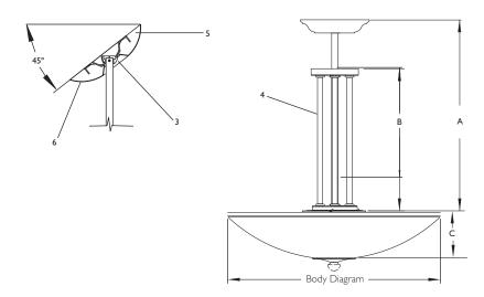
Complete Luminaire consists of Body and Suspension. Order each separately. Multiple Stem Suspension, with Swivel, Traditional Canopy.
