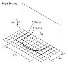
Average initial footcandles = 3.11 Maximum initial footcandles = 10.1 Minimum initial footcandles = 0.4 Maximum to minimum ratio = 25.25
