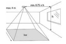
Sensor should be located where it sees a combination of Electric light and Daylight.
