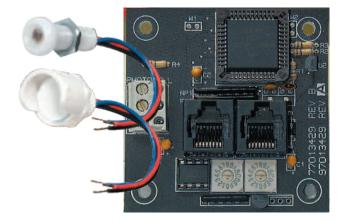
Network photo sensor controller Indoor and outdoor sensor
