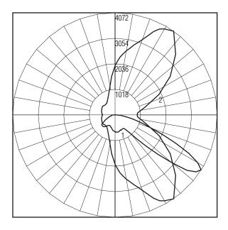
SQUARE CANOPY LIGHT - 49 LED BOARD - TYPE 2 WITH TYPE 3 LED FREEFORM LENS OPTICS AND CLEAR PRISMATIC POLYCARBONATE DOME LENS 49 WHITE LEDS. LUMEN OUTPUT = 4930 LMS.
