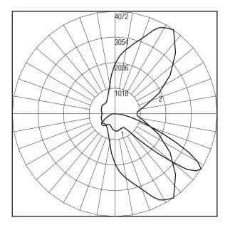
SQUARE CANOPY LIGHT - 49 LED BOARD - TYPE 3 WITH INDIVIDUAL LED FREEFORM LENS OPTICS AND CLEAR PRISMATIC POLYCARBONATE DOME LENS 49 WHITE LEDS. LUMEN OUTPUT = 4891 LMS.
