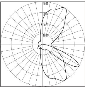
MCL ROADWAY LED OUTDOOR AREA LIGHT - TYPE III WITH INTERNAL ACRYLIC COLLUMATOR AND FLAT GLASS LENS 54 WHITE LEDS. LUMEN OUTPUT = 4395 LMS.
