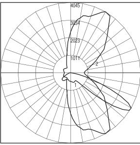
SILHOUETTE ROADWAY LED OUTDOOR AREA LIGHT - TYPE III WITH INTERNAL ACRYLIC COLLUMATOR AND FLAT GLASS LENS 54 WHITE LEDS. LUMEN OUTPUT = 4395 LMS.
