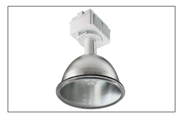
nect plug provided fro connection to input supply wires. Prewired high power factor ballast designed for up to 55°C ambient temperatures, -29°C starting temperature for Metal Halide and -40°C for HPS. Encapsulated in polyester resin compound with capacitors and ignitors located outside encapsulation. Lamp current crest factor less than 1.65.
